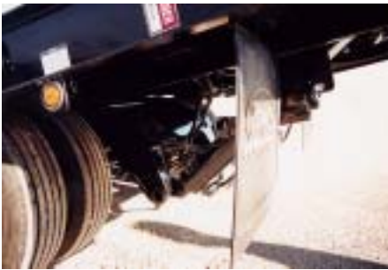
Heavy duty Etnyre folding tail design.
